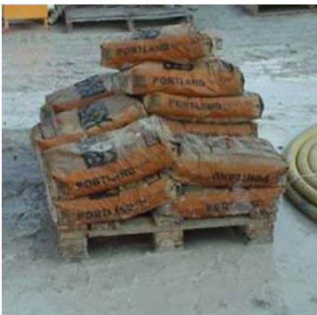
Water-logged pallet of cement bags
